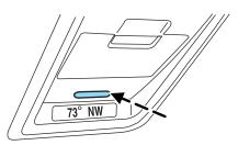
If the outside temperature falls below 3°C (38°F), the display will alternate from "ICE" to the outside temperature at a two second rate for one minute.
